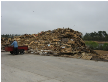
Lumber and pallets are stored on one corner of the New Hanover County landfill C&D pad until the material is scheduled for grinding.
